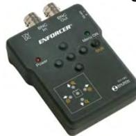
Use to access the OSD (On-Screen Display) functions for compatible cameras without having to be near the camera.
