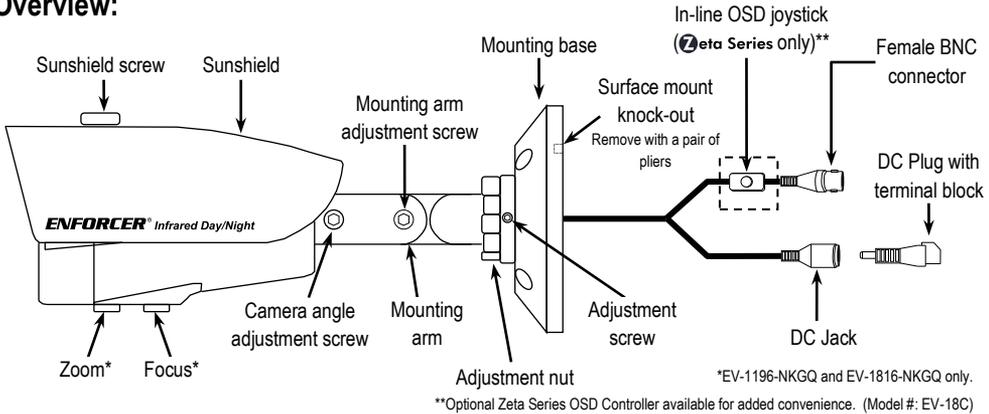
ENFORCER IR LED Bullet Cameras can be mounted to a standard lamp holder cover plate (not included).
