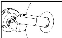
The mounting arm set screws can be loosened in two places to adjust the camera angle. The adjustment ring at the base can also be adjusted.
