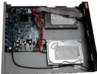
5. Each hard drive requires 4 screws to be properly secured to the DVR frame. Secure each hard drive to the DVR using the included screws. Use 2 screws to secure one side of a hard drive to the DVR as shown.
