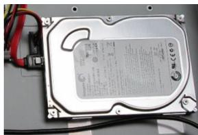
9. Locate the power connectors. Connect one power connector to each hard drive.
