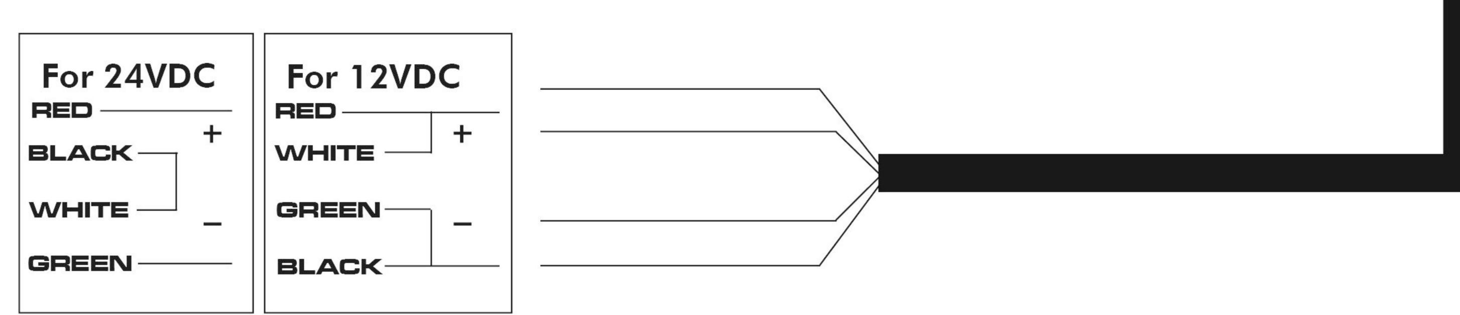
Before applying power, check the wire connections. Incorrect connections may result in a burned-out electromagnet.
