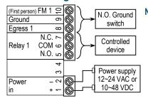
NOTE: The *first person-in* (first-man-in, FM) function suspends the timer operation when its optional N.O. switch is activated. If the corresponding relay is turned on before *FM* switch is activated, the relay remains on until the *FM* switch is deactivated. Once deactivated, the timer turns on the last programmed function prior to *FM* activation.
