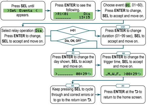
**NOTE**: Relay operations are Dis (shunt), ON, t=x (momentary, where x=01~99 seconds), or OFF.
