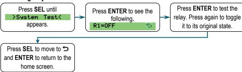
**NOTE:** Performing the system test toggles the relay based on its current state. If it is currently ON, pressing ENTER to test will toggle it OFF and vice versa.
