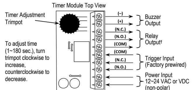
**\*IMPORTANT:** For 24VDC operation, use the included 680Ω, 0.5W resistor in line with the red wire or the black wire.
