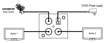
Max. range between camera and monitor determined by camera's max. distance
