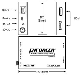
\*Transmitter and Receiver unit have the same dimensions †Input/Output are reversed on receiver
