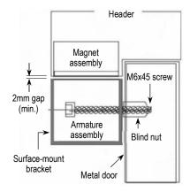
The magnet assembly is flush to the door frame or header and the armature assembly is in the bracket on the door.
