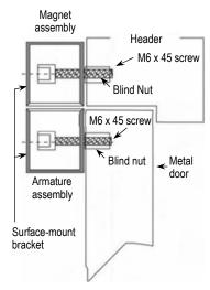
The magnet assembly is in the bracket above the door and the armature assembly is in the bracket on the door.
