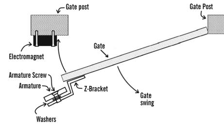
FIG. 3 - Installation on a double-swing gate
