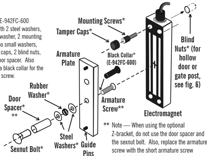
\*\* Note — When using the optional Z-bracket, do not use the door spacer and the sexnut bolt. Also, replace the armature screw with the short armature screw included with the bracket, or cover the exposed end of the long screw with the nut.
