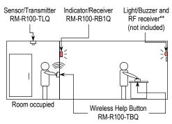
Room occupied - remote indicator/receiver LED is lit.
