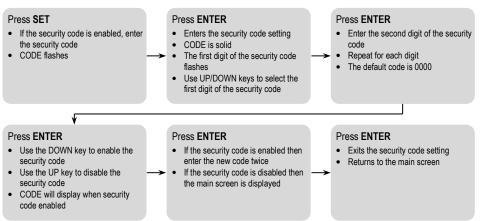
**Security Code Reset:** To reset the security code to the factory default (0000), press and hold the SET, ENTER, UP & DOWN keys for 3 seconds.
