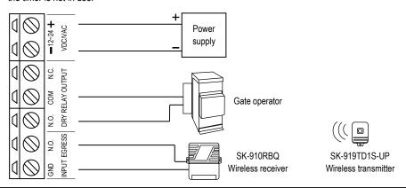
In this application, the SA-027WQ is used to keep an entry door unlocked during normal business hours. The door is to be left unlocked from 8:00am to 5:00pm Monday through Friday.
