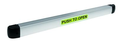
The ENFORCER Illuminated Push-to-Open Bar works with an external electric strike or maglock to provide egress from a protected area. It can work in stand-alone mode or as part of an access control system, but also can be locked open by key. Buzzer, output timing, and LED function and colors are also customizable.
