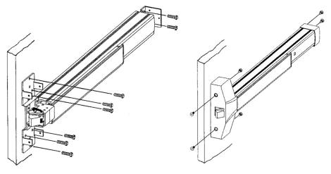
NOTE: Diagram shows 6 screws for mounting the chassis. Product only includes 4 screws. For best results, use 6 screws.
