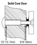
Drill an 5/16" (8mm) dia. hole on the door for the armature screw, and drill a 1/2" (12.7mm) dia. and 1" (25mm) deep hole for the sexnut screw.
