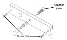
**Tip:** Use a thread-locking compound on the armature screw to ensure a long-lasting installation.
