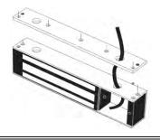
15. Cut the wires so they are long enough to connect with the terminal block. Set the voltage using the selection jumpers based on your input voltage.
