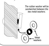
8. Tighten the armature screw enough so that the armature plate can withstand a break-in attempt, but loose enough so that the armature plate can pivot slightly. Make sure the anti-spin guide pins are in the two quide pin holes.
