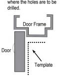
**4.** Drill two holes in the frame and three holes in the door as shown on the template.
