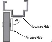
Magnet can be reversed depending on whether it is used for right-swing or left-swing doors.
