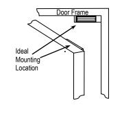
**3.** Place the template against the door and frame. Mark where the holes are to be drilled.
