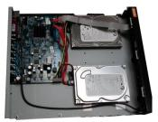
Once the side of the hard drive is secured to the DVR, use 2 screws to secure the bottom of the hard drive to the DVR as shown.
