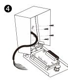
4. Mount the Housing Push wires through the hole in the housing back and mount to wall or post.
