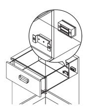
Mounting the maglock to the cabinet back (with or without the L-bracket) and the armature to the drawer back with the armature holder
