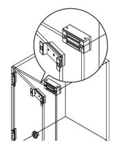
Mounting the maglock to the cabinet frame and the armature to the door with the armature holder
