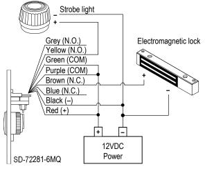
\*The sample application shown is an example of a momentary output. If a maintained output is required, then use the SD-72231-6MQ instead.
